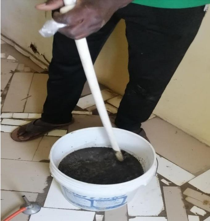
*Cow dung & water being stirred to be fed into the digester fermentation*
