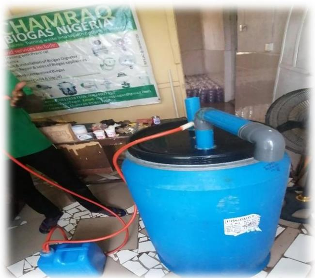
*a continuous biodigester system constructed during the training*
